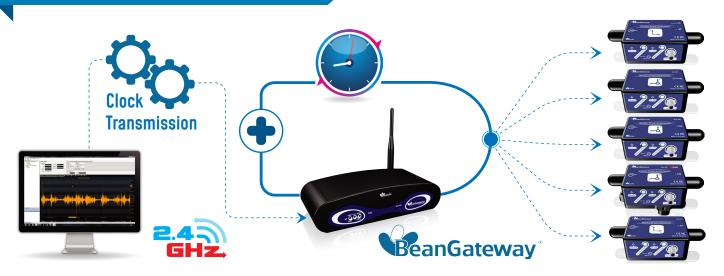
TimeSync function brings time-synchronization over the Wireless IIOT Sensors (±2.5ms of accuracy between each Wireless IIOT Sensors) and contributes to enhance user experience about correlation of remote sensing data and modal analysis
