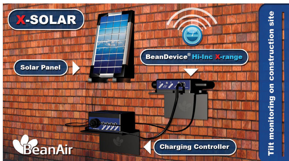
Caption 3: The wireless tilt sensor can monitor tilt on both horizontal direction with an accuracy of \pm 0.05^\circ and a resolution of \pm 0.001^\circ
