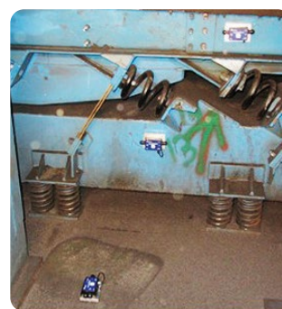
Caption 1: Floor vibration measurement: Beandevic ® 2.4GHz AX-3D ±2G
