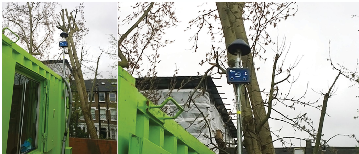
Caption 2: Mounted on a pole, the BeanGateway® 2.4GHz [outdoor version] can reach a wireless range of 300 meters in urban and noisy environment.
