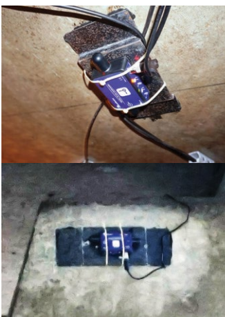
Caption 4: Wireless vibration sensors are used to extract resonance frequencies on Bridge Structure
