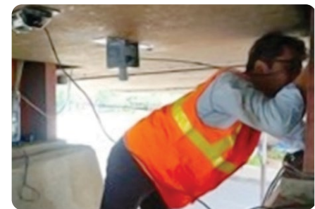
Caption 2: Laser sensor mounted with our wireless DAQ system [ref: BeanDevice® 2.4GHz AN-420 ]
