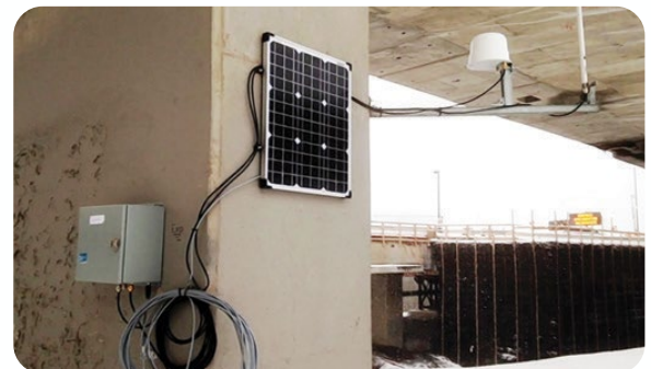
Caption 4: Wireless IIOT sensors Gateway with 4G connectivity enables remote access (Ref: BeanGateway® 2.4GHz 4G)
