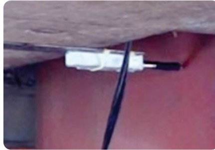
Caption 1: LVDT sensor mounted with our BeanDevice® 2.4GHz AN-420
