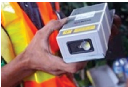
Caption 2: Laser sensor mounted with our wireless DAQ system [ref: BeanDevice® 2.4GHz AN-420 ]
