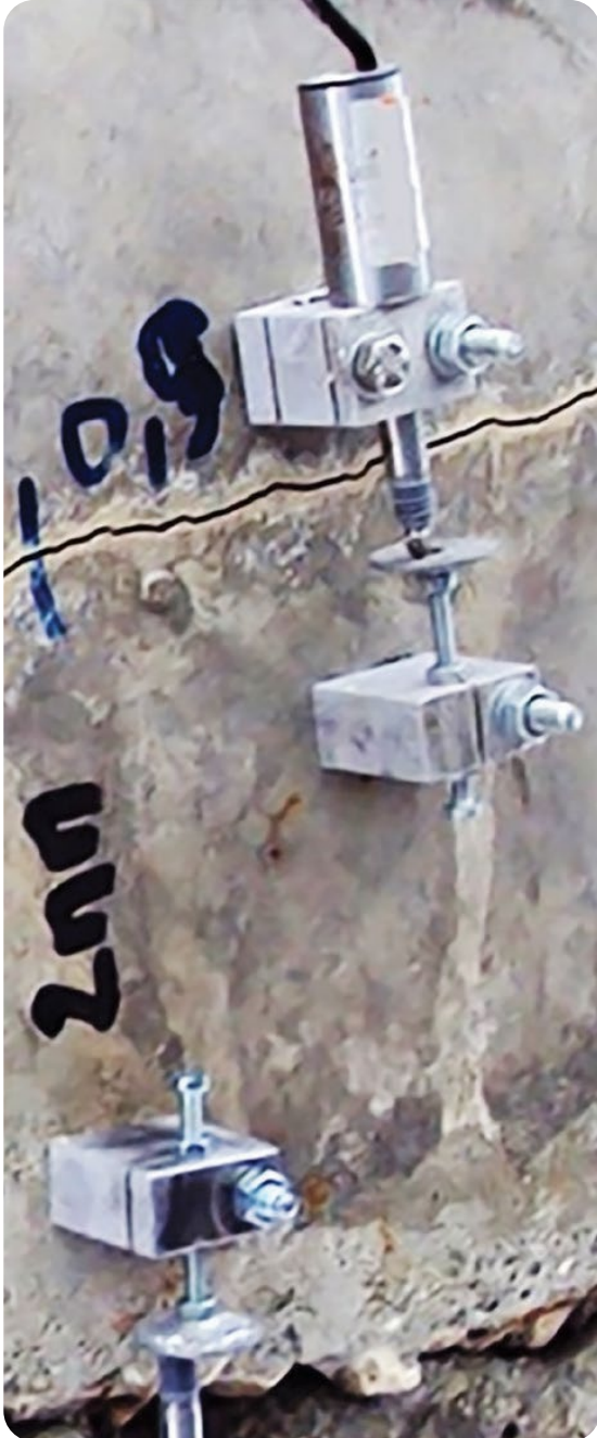
Caption 5: Displacement sensors are connected to our Wireless DAQ System (Ref: BeanDevice® 2.4GHz AN-mV)
