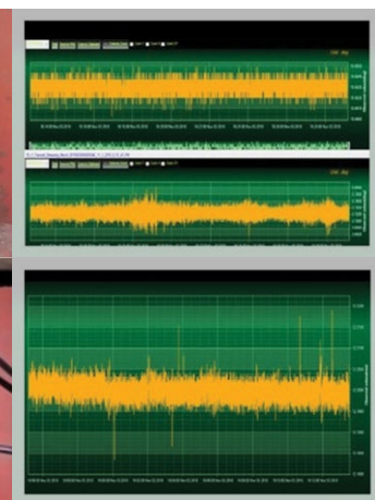
Caption 4: Wireless vibration sensors are used to extract resonance frequencies on Bridge Structure
