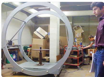
Caption 12: Magnetic field testing
