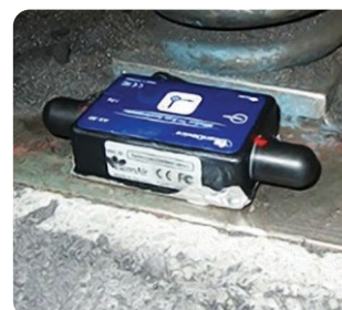
Caption 2: Conveyors machines are monitored with our wireless accelerometers [Ref: Beandevic ® 2.4GHz AX-3D]
