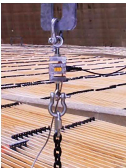
Caption 5: Load cell is connected to a Wireless DAQ (BeanDevice® 2.4GHz AN-mV)
