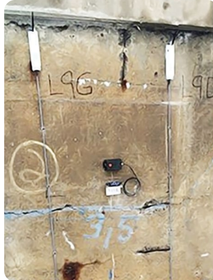
Caption 6: Wireless Inclinometers mounted on a 90° mounting bracket (Ref: BeanDevice® 2.4GHz HI-INC) are used to monitor the concrete structure
