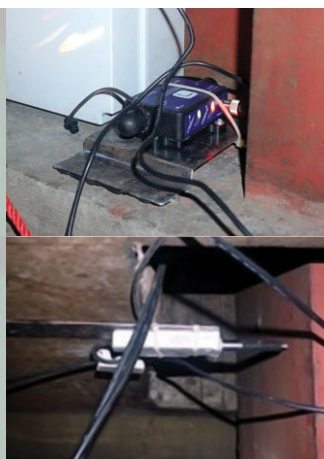
Caption 4: Wireless vibration sensors are used to extract resonance frequencies on Bridge Structure
