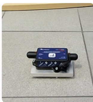
Caption 1: Floor vibration measurement: Beandevic ® 2.4GHz AX-3D ±2G
