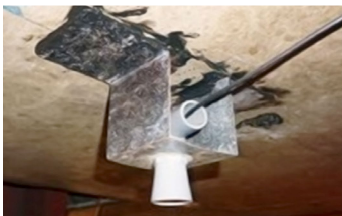
Caption 5: Connected to our Wireless DAQ System [ Ref: BeanDevice® 2.4GHz AN-V ) , the ultrasonic sensor is used to measure bridge movement.
