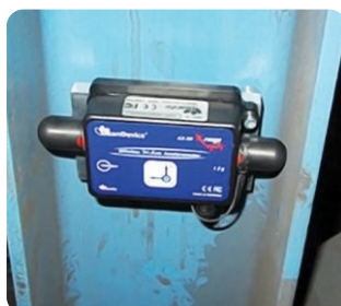
Caption 2: Conveyors machines are monitored with our wireless accelerometers [Ref: Beandevic ® 2.4GHz AX-3D]
