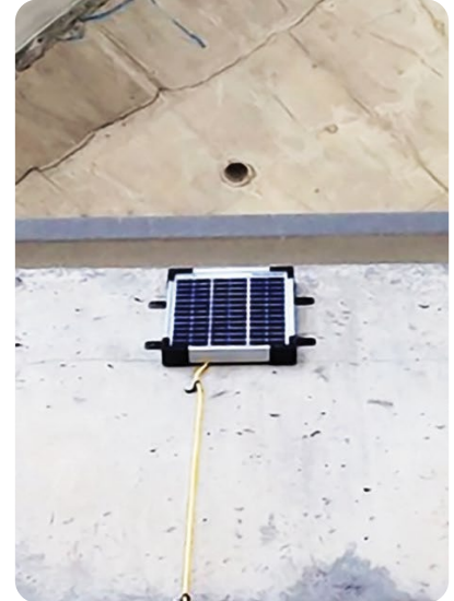
Caption 7: A 10W Solar Panel is powering 4 Wireless Inclinometers at the same time (Ref: BeanDevice® 2.4GHz HI-INC)
