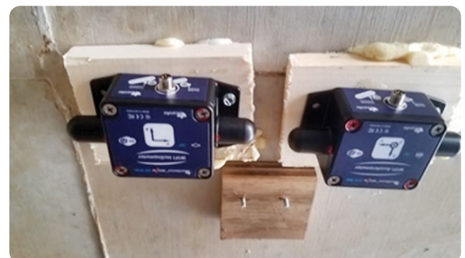
Caption 15: Wireless vibration sensors mounted with screws
