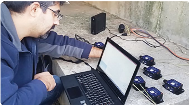
Caption 12: Deployment of 10 wireless vibration sensors (Ref: BeanDevice® Wilow® AX-3D \pm 2g )
