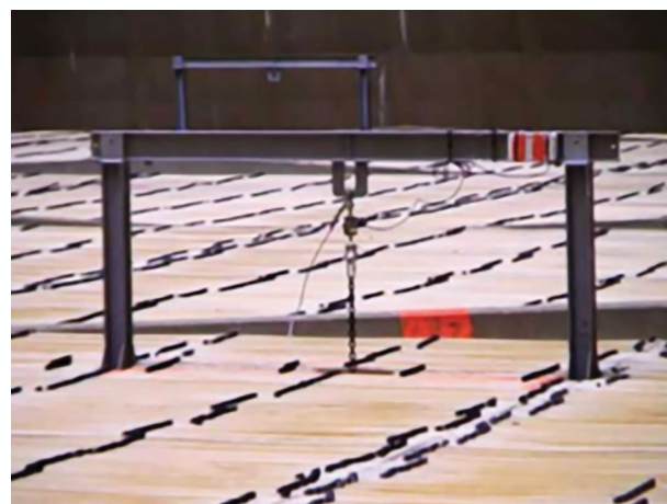
Caption 4: Load cell is used to monitor fill packing weight (counterflow water/air)
