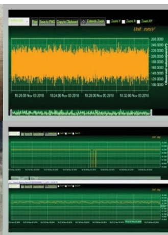
Caption 4: Wireless vibration sensors are used to extract resonance frequencies on Bridge Structure
