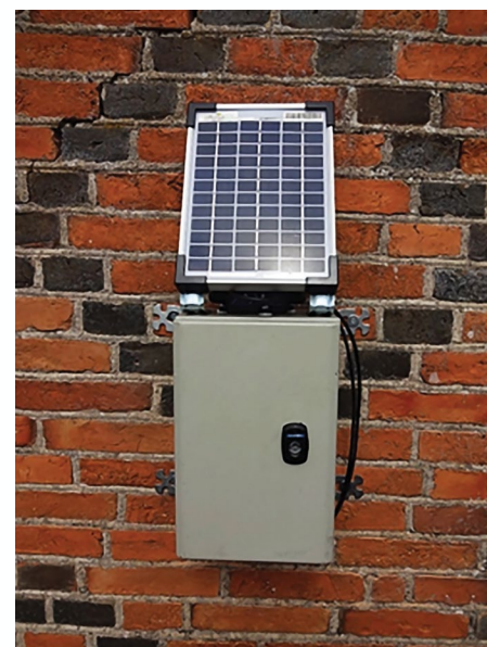
Caption 4: Wireless tiltmeter (Ref: Beandevic® 2.4GHz HI-INC Xrange) is mounted on the noise barrier (brick construction)
