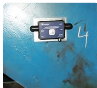
Caption 2: Conveyors machines are monitored with our wireless accelerometers [Ref: Beandevic ® 2.4GHz AX-3D]
