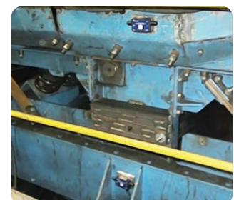
Caption 2: Conveyors machines are monitored with our wireless accelerometers [Ref: Beandevic ® 2.4GHz AX-3D]
