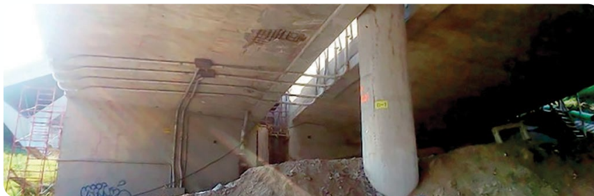
Caption 2: Wireless inclinometers are screw mounted on pillars
