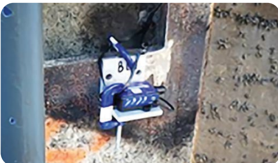
Caption 3: Wireless vibration sensors mounted on a concrete structure with a 90° mounting bracket (Ref: BeanDevice® 2.4GHz AX-3D)
